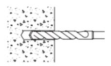
1. Using the proper diameter bit, drill a hole into the base material to a depth of at least 1/4" deeper than the required embedment. The tolerances of the drill bit used should meet the requirements of ANSI Standard B212.15. Blow the hole clean of dust and other material.
