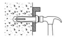
2. Insert the anchor through the fixture and into the drilled hole. Drive the nail into the anchor body to expand it. Be sure the head is seated firmly against the fixture and that the anchor is the proper embedment. Take care not to overdrive the nail. This anchor is not recommended for installations at an angle or use overhead.
