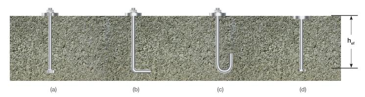
Cast-in anchors: (a) hex head bolt with washer; (b) L-bolt; (c) J-bolt; (d) welded headed stud.
