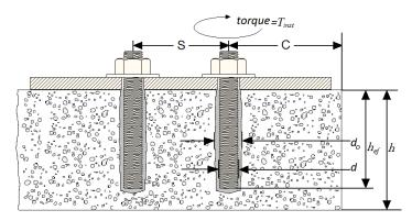
FIGURE 2—TYPICAL INSTALLATION DETAIL FOR THREADED RODS AND REINFORCING BARS
