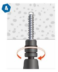
4. Install the anchor with an impact wrench through the surface. The correct force should be considered during the installation to make sure the socket doesn't do damage to the member surface or self-inflict any dmagae to its connecting threads.
