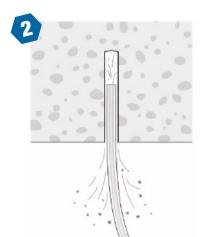
2. Remove dust and debris from the hole using a hand pump or compressed air.
