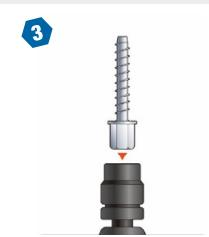
3. Select a powered impact wrench of a torque wrench, attach an appropriate sized hex socket to the wrench and mount the screw anchor head into the socket.
