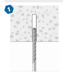
Drill a hole into the base material to the required depth using a drill bit that meets the requirements of ANSI B212.15.
